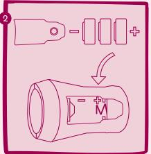
Install 3 x AG3 (1.5V) batteries and follow the polarity orientation, as shown.
