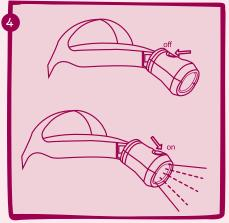
To activate light, slide switch to "ON"
