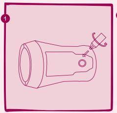
Open the battery cover with a screwdriver. (Phillips screwdriver not included)
