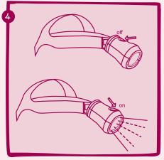
To activate light, slide switch to "ON"
