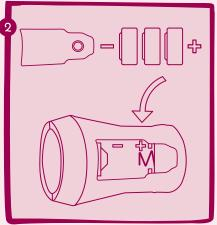
Install 3 x AG3 (1.5V) batteries and follow the polarity orientation, as shown.
