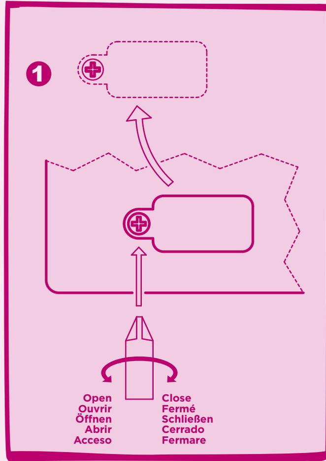
(EN): Open and close the battery cover with a screwdriver (Philips screwdriver not included).
