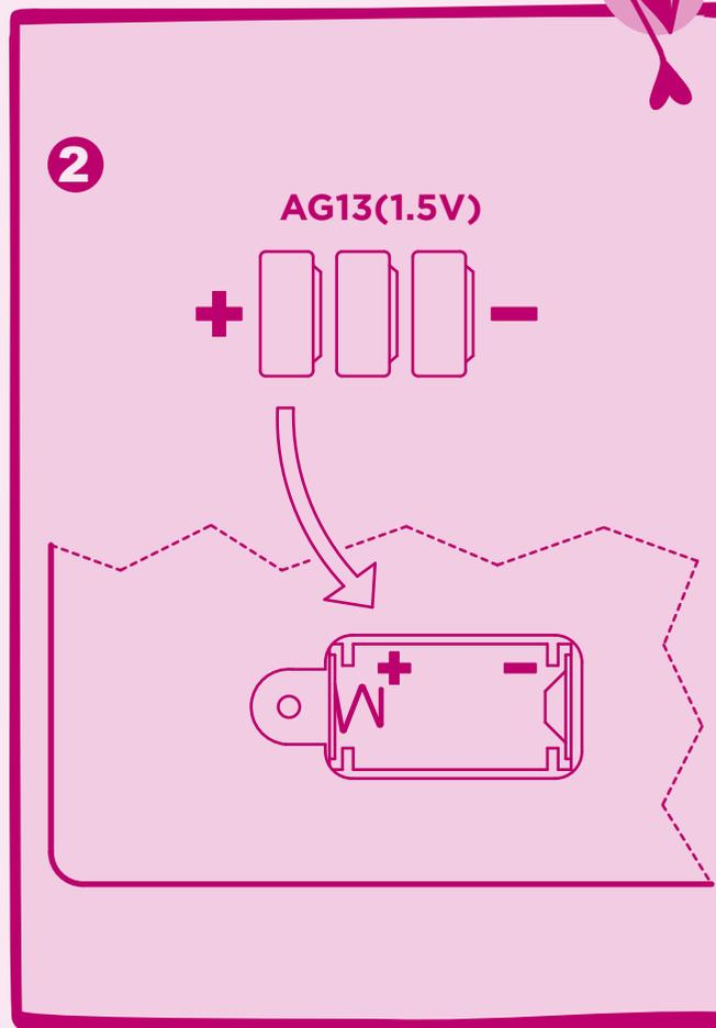
(EN): Install 3 x AG13 (1.5V) batteries and follow the polarity as shown.
