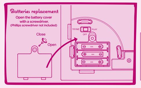
ATTENTION: When the module's functions lose performance, follow instructions carefully to install new batteries.
