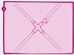
Place the cross joint at the top center of the tent and insert the poles, as shown.
