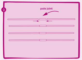
Assemble 2 poles with a pole joint. Repeat 4 times to make 4 long poles.
