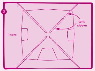
Insert the assembled poles into the sleeves of the tent.
